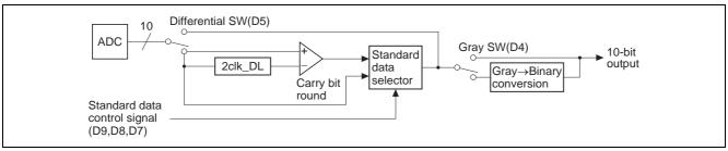
Figure 10 Differential Code, Gray Code Circuit
