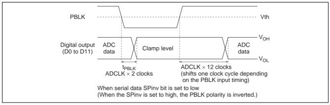
Figure 5 Detailed Timing Specifications at Pre-Blanking
