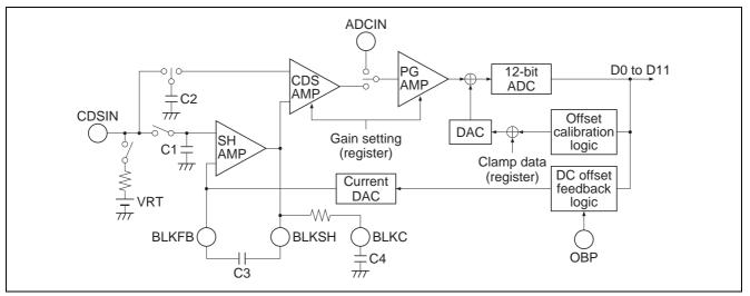
Figure 1 HD49338NP/HNP Functional Block Diagram
