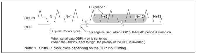
Figure 4 OBP Detailed Timing Specifications
