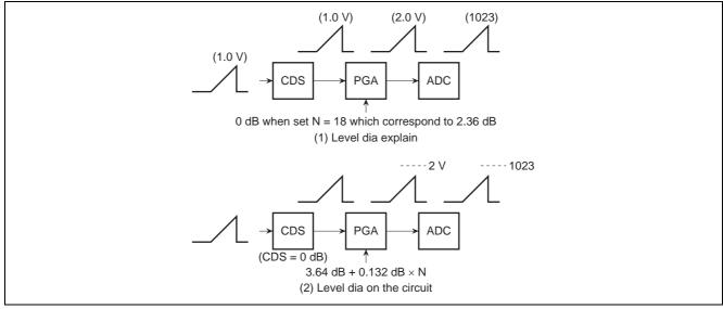
Figure 9 Level Dia of PGA
