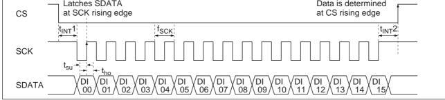
Figure 8 Serial Interface Timing Specifications
