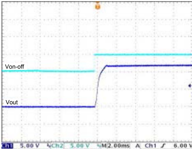
Graph 7: Using ON/OFF Voltage Start-Up and Vo Rise Characteristic (Nominal Vin and Full Load)
