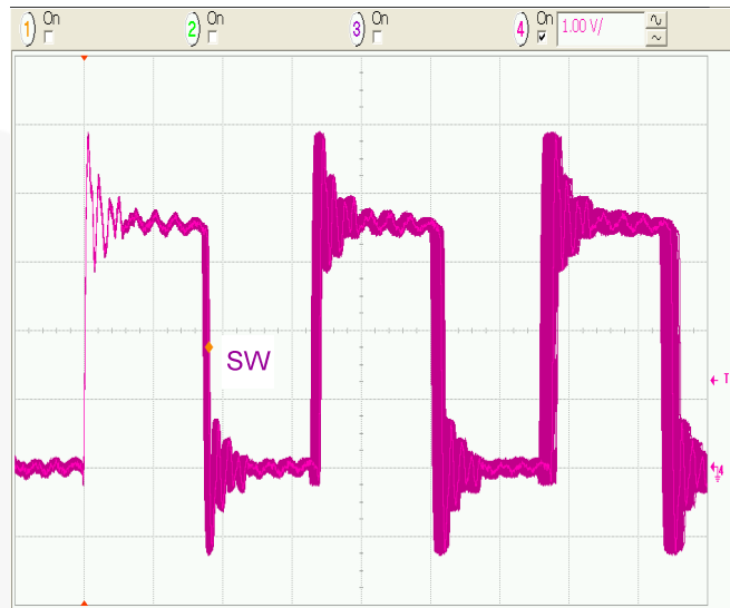
Figure 39. SW-Node Jitter (Infinite Persistence), I_{LOAD} = 200mA , 50ns/div .
