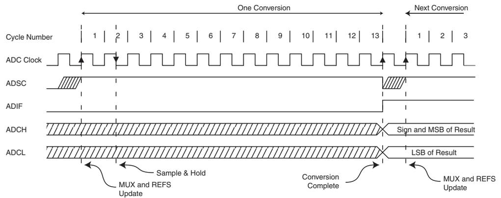
**Figure 23-6.** ADC Timing Diagram, Auto Triggered Conversion
