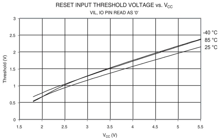
**Figure 29-32.** Reset Input Pin Hysteresis vs.  $V_{CC}$
