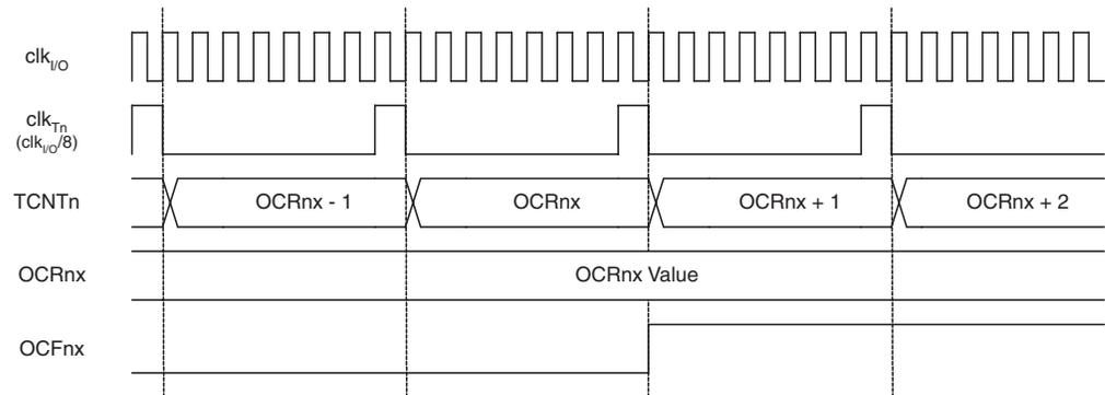
Figure 14-11 shows the setting of OCF0A and the clearing of TCNT0 in CTC mode and fast PWM mode where OCR0A is TOP.
