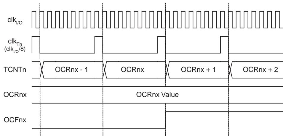
Figure 15-12 shows the count sequence close to TOP in various modes. When using phase and frequency correct PWM mode the  $OCR1x$  Register is updated at BOTTOM. The timing diagrams will be the same, but TOP should be replaced by BOTTOM, TOP-1 by BOTTOM+1 and so on. The same renaming applies for modes that set the TOV1 Flag at BOTTOM.
