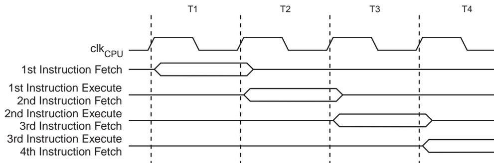
Figure 6-5 shows the internal timing concept for the Register File. In a single clock cycle an ALU operation using two register operands is executed, and the result is stored back to the destination register.
