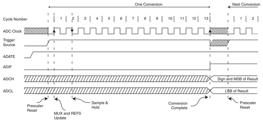
**Figure 23-7.** ADC Timing Diagram, Free Running Conversion
