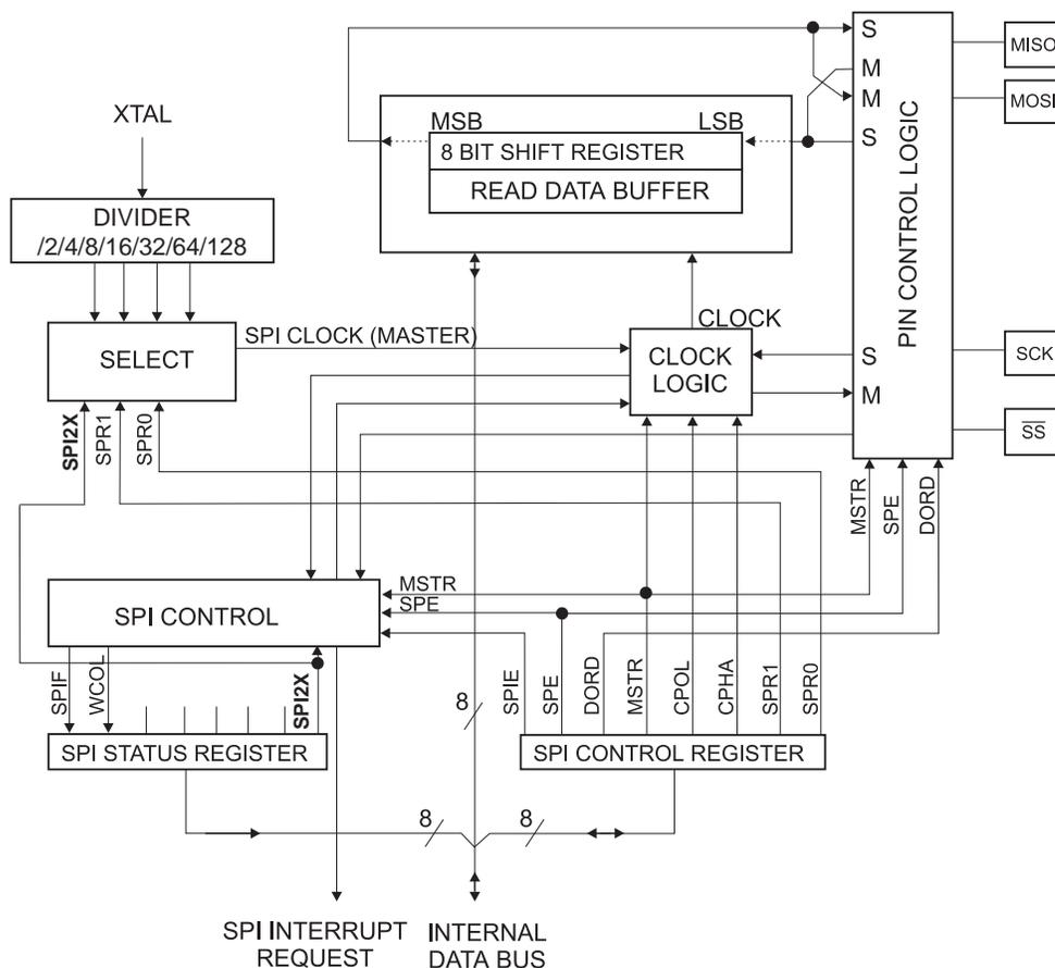
Note: 1. Refer to [Figure 1-1 on page 2](#), and [Table 13-3 on page 79](#) for SPI pin placement.
