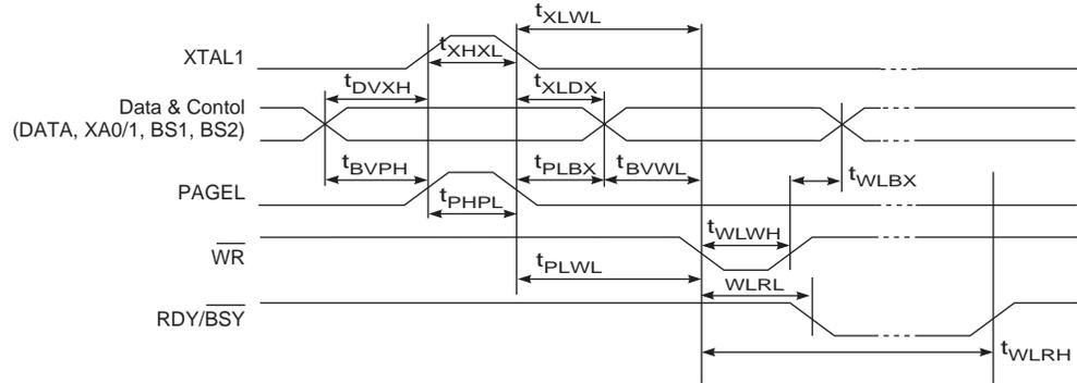
Figure 28-8. Parallel Programming Timing, Loading Sequence with Timing Requirements<sup>(1)</sup>
