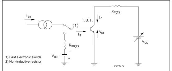
Figure 15. Energy rating test circuit
