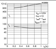
Figure 12. Resistive load switching off Figure 13. Resistive load switching off times
