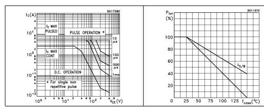
Figure 4. Output characteristics
