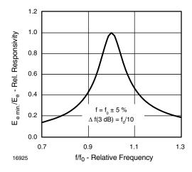
Fig. 5 - Frequency Dependence of Responsivity
