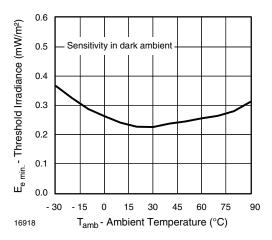
Fig. 10 - Sensitivity vs. Ambient Temperature
