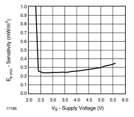
Fig. 13 - Sensitivity vs. Supply Voltage
