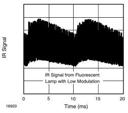
Fig. 14 - IR Signal from Fluorescent Lamp with Low Modulation
