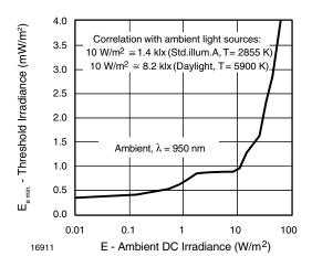
Fig. 6 - Sensitivity in Bright Ambient
