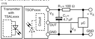
$\rm R_1$  and  $\rm C_1$  recommended to suppress power supply disturbances. The output voltage should not be hold continuously at a voltage below  $\rm V_o$  = 2.0 V by the external circuit.
