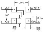
Bypass capacitor, C-by, should be ceramic capacitor ≥ .01uf.
