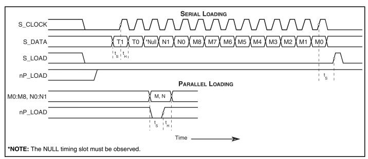
Figure 1. Parallel & Serial Load Operations
