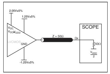
3.3V/2.5V LVPECL Output Load AC Test Circuit
