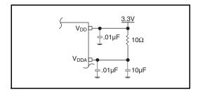
Figure 2. Power Supply Filtering
