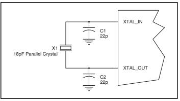
Figure 3. Crystal Input Interface
