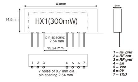
Figure 3: HX1 pin-out and dimension
