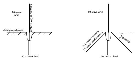
Fig.5: Quarter wave antenna / ground plane configurations
