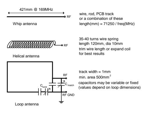
Figure 4: integral antenna configurations
