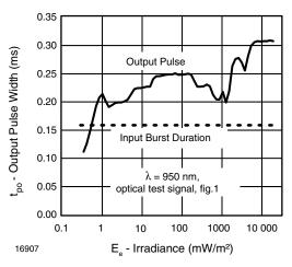
Fig. 2 - Pulse Length and Sensitivity in Dark Ambient
