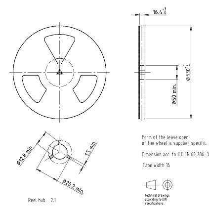
Drawing refers to following types: Reel for blister carrier tape Version B Drawing-No.: 9.800-5052.V2-4 Issue: 1; 07.05.02
