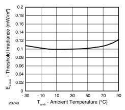
Fig. 10 - Sensitivity vs. Ambient Temperature
