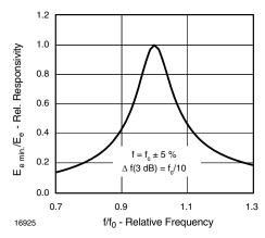
Fig. 5 - Frequency Dependence of Responsivity
