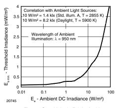
Fig. 6 - Sensitivity in Bright Ambient
