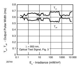
Fig. 4 - Output Pulse Diagram
