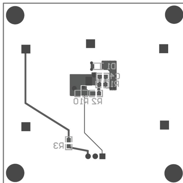
**Figure 4: AAT1218 Evaluation Board Bottom Side Layout.**
