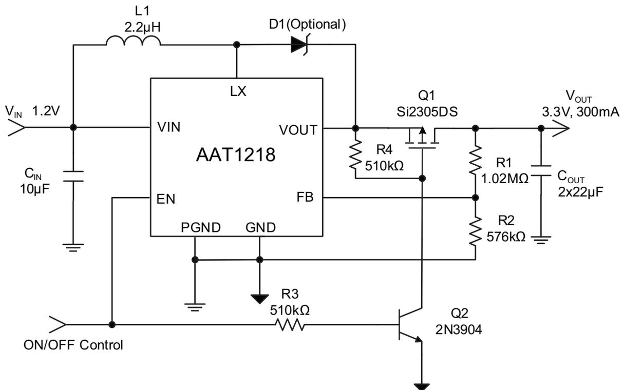
**Figure 1: AAT1218 Application Schematic with Load Disconnect Circuit.**
