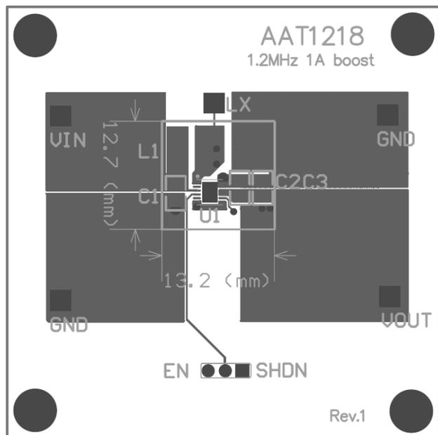
**Figure 3: AAT1218 Evaluation Board Top Side Layout.**
