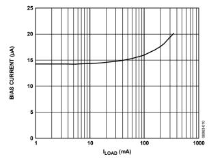
Figure 10. Bias Current vs. Load Current
