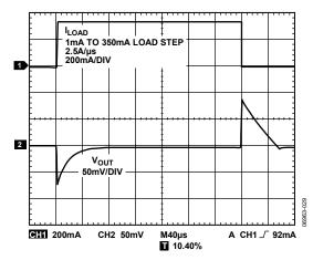
Figure 29. Load Transient Response
