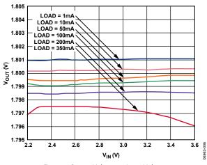
Figure 6. Output Voltage vs. Input Voltage
