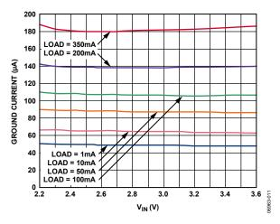
Figure 11. Ground Current vs. Input Voltage
