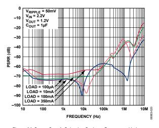
Figure 20. Power Supply Rejection Ratio vs. Frequency, V<sub>IN</sub> Input
