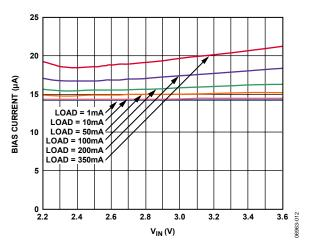
Figure 12. Bias Current vs. Input Voltage
