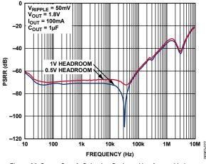
Figure 22. Power Supply Rejection Ratio vs. Headroom, VIN Input
