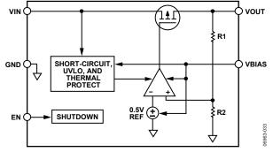
Figure 33. Internal Block Diagram
