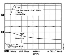
Figure 35. Output Transient Response,  $C_{OUT} = 10 \, \mu F$
