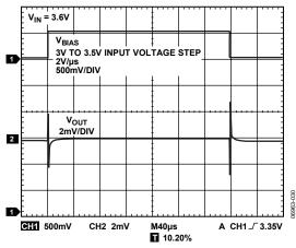
Figure 30. V<sub>BIAS</sub> Line Transient Response, V<sub>IN</sub> = 3.6 V, I<sub>OUT</sub> = 350 mA
