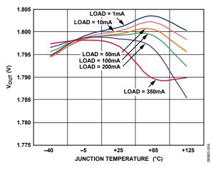
Figure 4. Output Voltage vs. Junction Temperature
