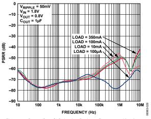
Figure 26. Power Supply Rejection Ratio vs. Frequency,  $V_{\text{BIAS}}$  Input
