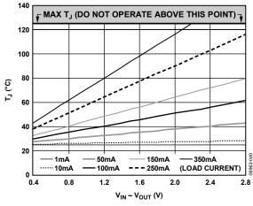
Figure 40. 500 mm<sup>2</sup> of PCB Copper,  $T_A = 25^{\circ}$ C, TSOT
