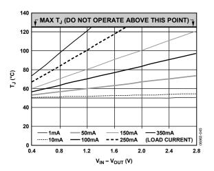
Figure 45. 0 mm<sup>2</sup> of PCB Copper,  $T_A = 50^{\circ}$ C, TSOT
