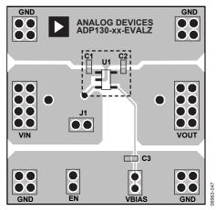
Figure 47. Example TSOT PCB Layout
