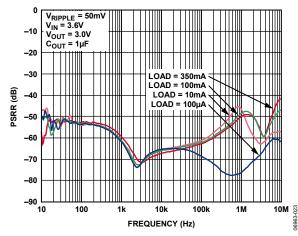
Figure 23. Power Supply Rejection Ratio vs. Frequency, V<sub>BIAS</sub> Input
