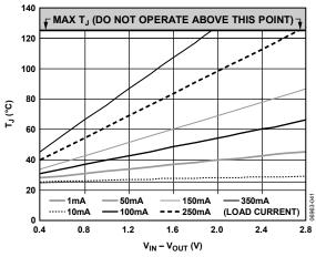
Figure 41. 100 mm<sup>2</sup> of PCB Copper,  $T_A = 25^{\circ}C$ , TSOT
