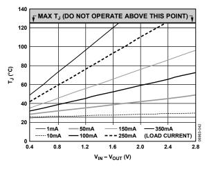
Figure 42. 0 mm<sup>2</sup> of PCB Copper,  $T_A = 25$ °C, TSOT
