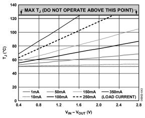
Figure 43. 500 mm<sup>2</sup> of PCB Copper,  $T_A = 50^{\circ}$ C, TSOT
