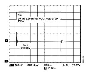
Figure 31. V<sub>IN</sub> Line Transient Response, V<sub>BIAS</sub> = 5 V, I<sub>OUT</sub> = 1 mA
