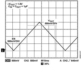
Figure 37. Typical EN Pin Operation
