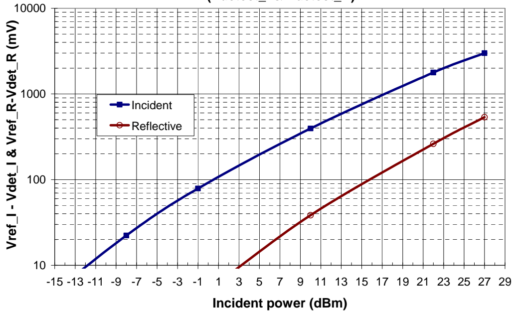
Incident and reflective power detection versus Incident power @ 27GHz (Vdetect_I & Vdetect_R)
