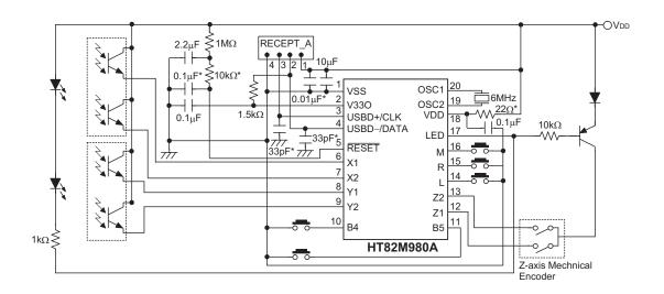
Note: Layout  $0.1\mu F$  capacitor,  $22\Omega$  resistor and  $0.01\mu F$  capacitor as close to VDD pin as possible.
