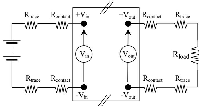
**Output Ripple Voltage Setup**
