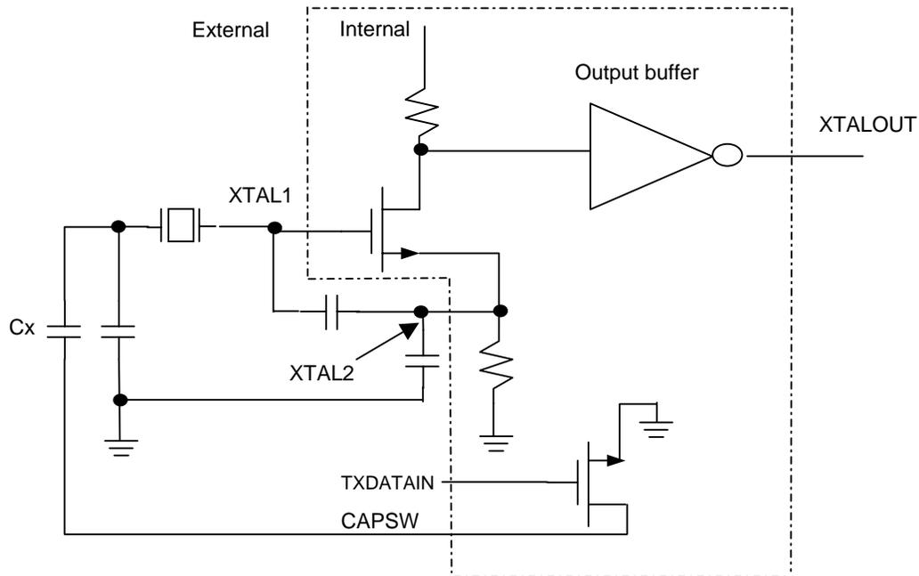
Figure 8. Crystal Oscillator and FSK modulation Circuit
