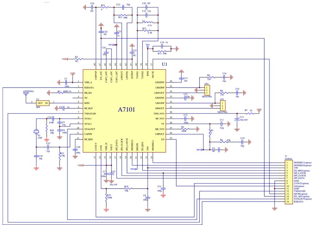
Figure 10. Application Circuit for Transceiver (Data rate = 64Kbps)
