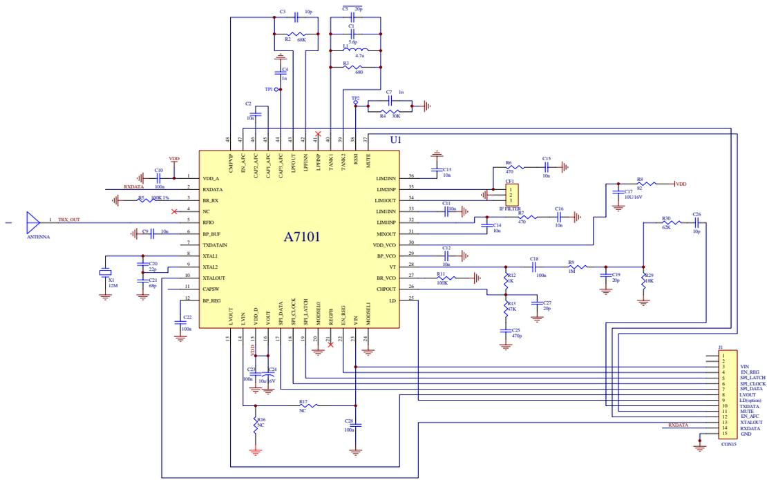
Figure 11. Application Circuit for Transceiver (Data rate = 250Kbps)
