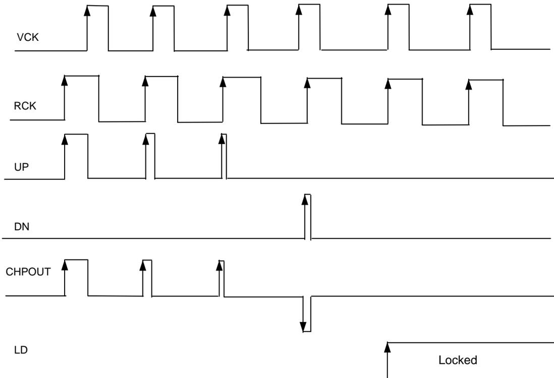
Figure 7. The PFD output waveform
