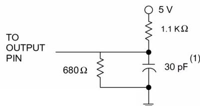
Note: 1. Includes jig and scope capacitance.
