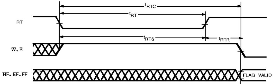
Note: 1.  $\overline{EF}$ ,  $\overline{FF}$  and  $\overline{PHF}$  may change status during Retransmit, but flags will be valid at  $t_{RTC}$
