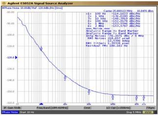
Phase noise of the reference signal, Out1. 25MHz Reference Frequency
