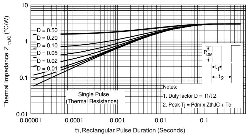
Fig. 4 - Maximum Thermal Impedance  $Z_{thJC}$  Characteristics
