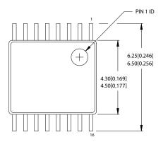
Figure 8. 16-lead TSSOP 4.40 MM Body Z16.173
