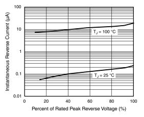
Figure 4. Typical Reverse Leakage Characteristics Per Diode
