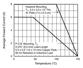
Figure 1. Derating Curve Output Rectified Current
