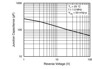
Figure 5. Typical Junction Capacitance Per Diode
