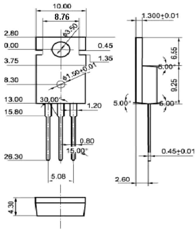
**Fig.2 Outline dimensions (unindicated tolerance:  $\pm 0.10\text{mm}$ )**
