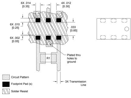
Dimensions are in Inches [Millimeters] Mounting Footprint
