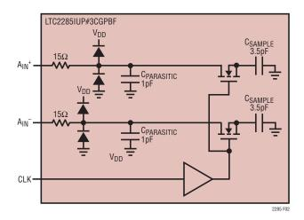
Figure 2. Equivalent Input Circuit
