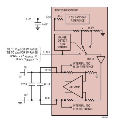
Figure 9. Equivalent Reference Circuit
