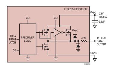
Figure 14. Digital Output Buffer
