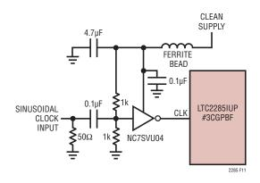
Figure 11. Sinusoidal Single-Ended CLK Drive
