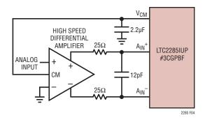
Figure 4. Differential Drive with an Amplifier
