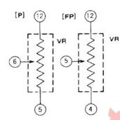
M5290P, FP is fixed the tracking voltage by inside resistor, but user can adjust it by using the output resistor. (inside resistor: ② to ⑥ ⑥ to ⑤,  $10k\Omega$  for the M5290P): ③ to ⑤ ⑤ to ④,  $10k\Omega$  for the M5290FP
