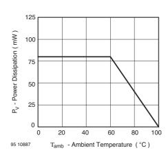
Figure 1. Power Dissipation vs. Ambient Temperature
