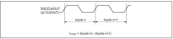
Figure 1 Cycle to cycle jitter
