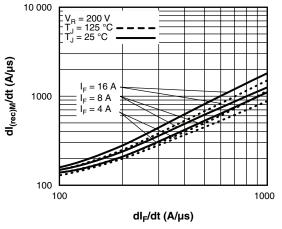
Fig. 8 - Typical dI<sub>(rec)M</sub>/dt vs. dI<sub>F</sub>/dt
