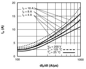
Fig. 6 - Typical Recovery Current vs. dI<sub>F</sub>/dt
