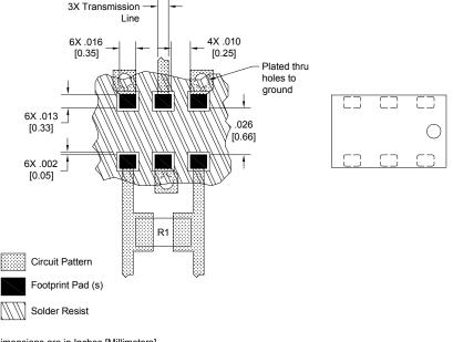
Dimensions are in Inches [Millimeters] Mounting Footprint
