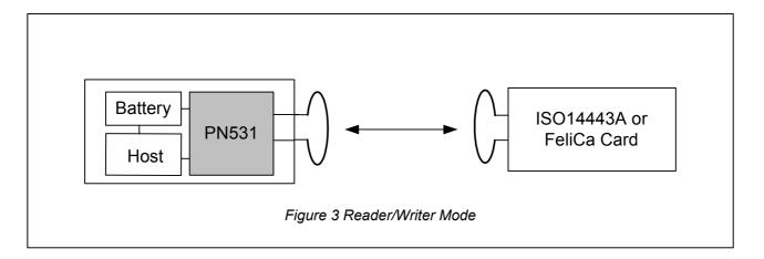
In the reader/ writer mode the PN531 enables communication to a passive ISO14443A/MIFARE® or FeliCa<sup>TM</sup> card
