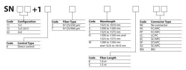
1. The 250  $\mu m$  fiber option is only available with the "no connector" option.
