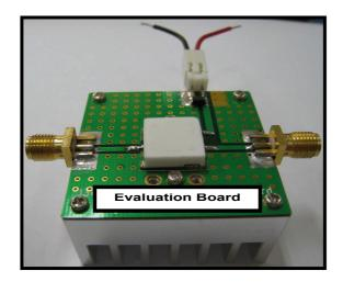
\* In order to prevent damage of D.U.T (APM-Series) from heating, you must to use a properly sized heat sink for testing a module.
