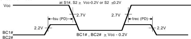
note11:On the S1# control mode, the level of S2 must be fixed
