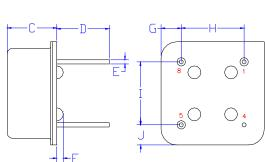
Cover: Kovar **Electroless Nickel Plated** 1 µinch (25 µm) typical Resistance welded to base
