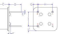
Cover: Kovar Electroless Nickel Plated 1 µinch (25 µm) typical Resistance welded to base
