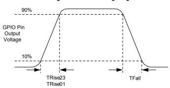
Figure 5. GPIO Timing Diagram
