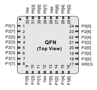
Table 1. 32-Pin Part Pinout (QFN)
