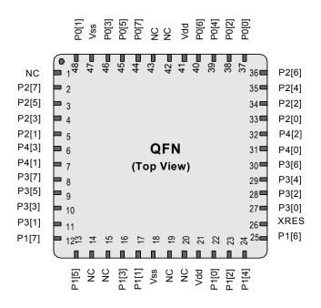
Table 2. 48-Pin Part Pinout (QFN)
