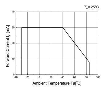
**Ambient Temperature vs. Forward Current**
