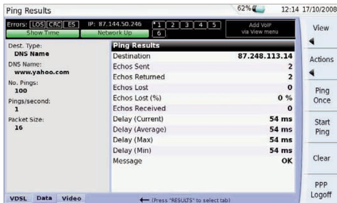
Figure 7: IP Ping test interface
