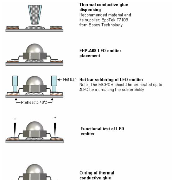
Handling Indications: Do not handle the EHP-A08 by the lens at any time during the assembly process. This can cause damage to the optical surfaces or may dislocate the lens if excessive force is applied.
