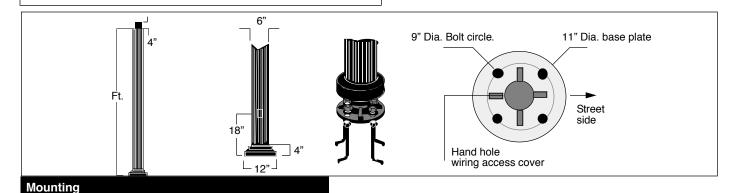
Base plate is provided with a 3 3/4" dia. opening for power entry . Galvanized anchor bolts : Set of 3/4-10 x 18" lg. anchor bolts.
