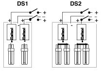
DS2: Luminaire ballast housing length and stem size may be increased to accomodate required number of ballasts.
