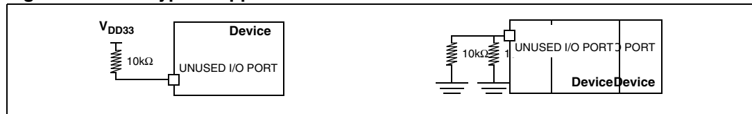
Figure 10. Two typical Applications with unused I/O Pin
