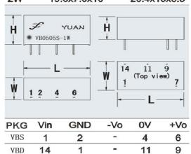
Note:PIN"7" can't connect any component.
