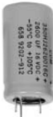
Type 350's solid aluminum top assures extremely low impedance. With a typical 4 to 6 nH ESL, the self resonant frequency is well above 100 kHz. The very low ESR assures the low impedance rating. The capacitors are fitted with three rugged welded mounting leads to provide maximum resistance
