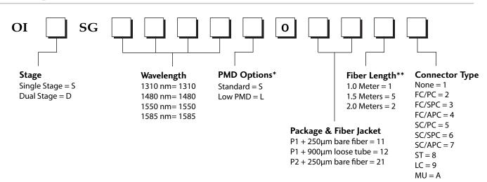
\*For OIDSG series, the PMD option is 'S'. For OISSG series, the PMD option is 'S' or 'L' based on customer's requirement. \*\*The tolerance of fiber length is +/-0.1m. 1 meter is standard. The lead-time for special fiber length will be longer.
