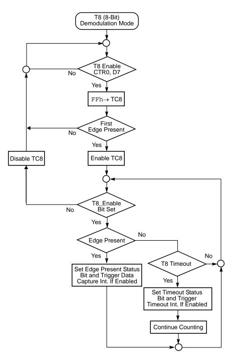
Figure 20. Demodulation Mode Flowchart
