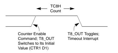
Figure 17. T8\_OUT in Single-Pass Mode
