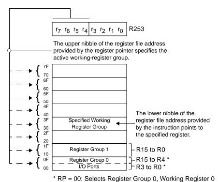
Figure 13. Register Pointer—Detail
