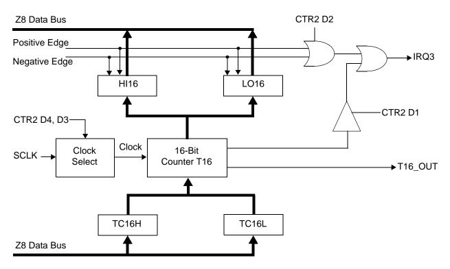
Figure 21. 16-Bit Counter/Timer Circuits
