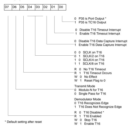
Figure 37. T16 Control Register ((0D) 2h: Read/Write Except Where Noted)
