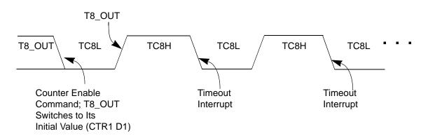
Figure 18. T8\_OUT in Modulo-N Mode
