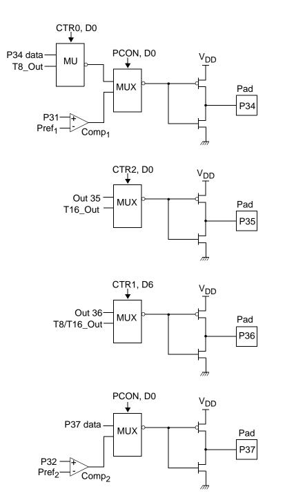
Figure 9. Port 3 Counter/Timer Output Configuration
