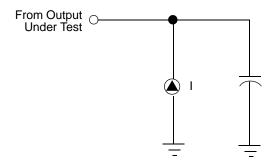
Figure 4. Test Load Diagram
