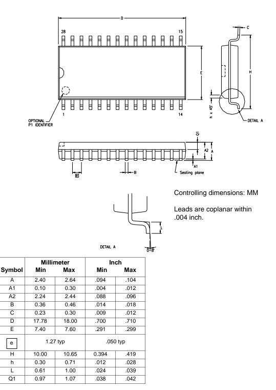
Figure 54. 28-Pin SOIC Package Diagram
