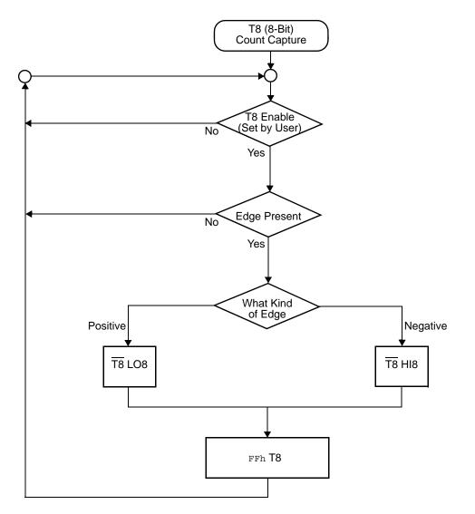
Figure 19. Demodulation Mode Count Capture Flowchart
