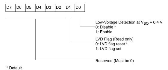
Figure 38. Low-Voltage Detection
