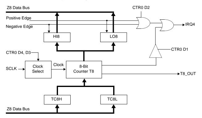
Figure 16. 8-Bit Counter/Timer Circuits
