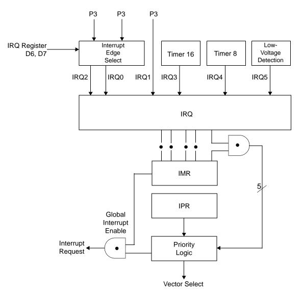
Figure 26. Interrupt Block Diagram
