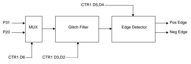
Figure 14. Glitch Filter Circuitry
