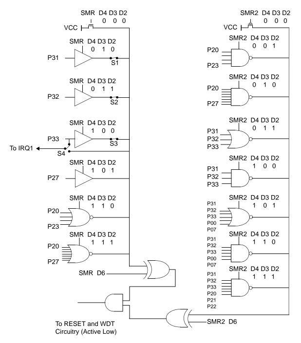
Figure 31. Stop-Mode Recovery Source
