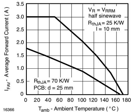
Figure 3. Max. Average Forward Current vs. Ambient Temperature
