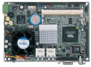
The HS-2607 is a 133MHz FSB VIA CLE266/VT8235 chipset-based board designed for Mini PCI Local Bus VIA Eden 1GHz Embedded CPU. These features combine and make the HS-2607 an ideal all-in-one industrial single board computer. Additional features include an enhanced I/O with CompactFlash reader, CRT/Panel, audio, dual LAN, TV-Out, 4 COM, and USB2.0 interfaces.
