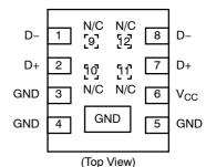
**\*NOTE:** Pins 1 and 9, Pins 2 and 10, Pins 7 and 11, Pins 8 and 12 are internally connected in pairs. It is recommended not to solder to Pins 9, 10, 11, 12.
